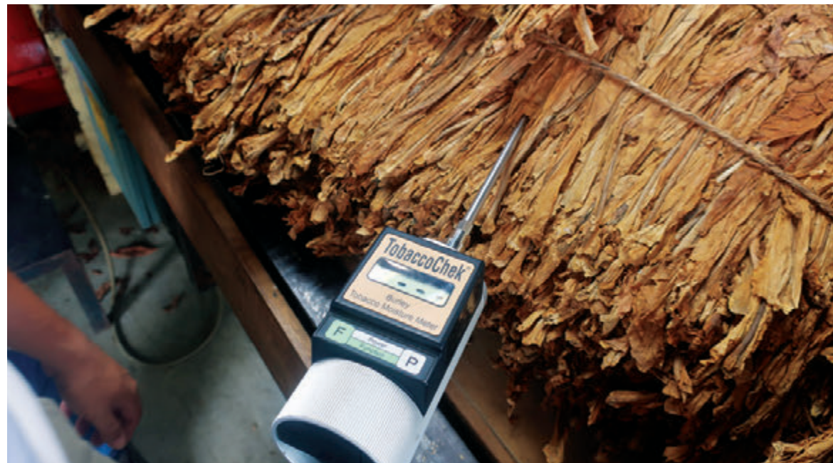
When receiving tobacco bales from farmers the tobacco is graded and moisture content is documented.
